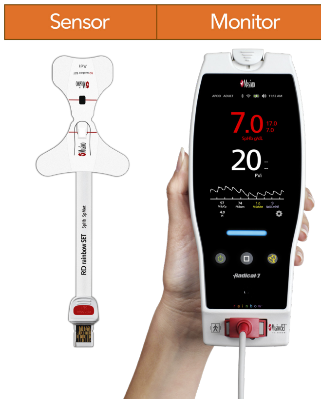
Figure 1 The figure shows the Masimo sensor (Masimo Rainbow Disposable Adhesive Sensor) and monitor (Masimo Radical-7, Masimo Corp, Irvine, California, USA). The sensor, placed on a finger hand, emits multiwavelength light. After passing through the measurement site, the light received by the photodetector generates electrical signals processed by advanced algorithms. The device provides an estimation of hemoglobin based on its absorbance characteristics. Furthermore, the device provides data about carboxyhemoglobin and methemoglobin concentration. SpHb, continuous non-invasive hemoglobin.
